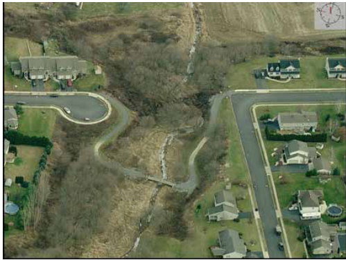
Sometimes streets dead end because of topographical barriers; pedestrian and bike paths can overcome these obstacles to connect communities.
