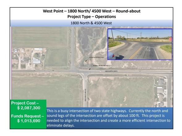
This intersection is at the crossroads of two very busy state highways. It is currently failing because the north and south legs are offset by 100'. It is already failing and new projects will bring additional traffic to the area. This intersection is adjacent to the future interchange of the West Davis Highway and SR37. The school district also owns property adjacent to this intersection and they plan to build an elementary, jr. high, and high school on the property.
