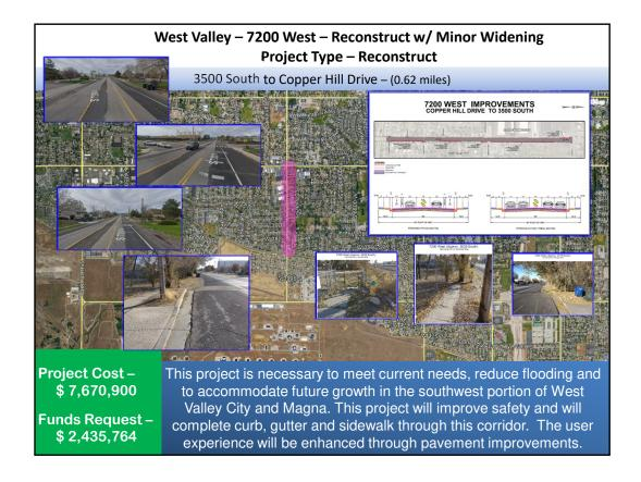
7200 West is a minor arterial serving both Magna and West Valley City and provides connectivity to two major East-West corridors (3500 South and 4100 South). This section of 7200 West is currently striped as a three-lane facility, with one thru lane each way and a two-way left turn median lane. This will be a partnership project between Magna Metro Township and West Valley City to reduce flooding and improve safety, mobility and user experience.
