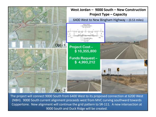
The project will connect 9000 South from 6400 West to its proposed connection at 6200 West (NBH). 9000 South current alignment proceeds west from MVC curving southward towards Coppertone. New alignment will continue the grid pattern to SR-111. A new intersection at 9000 South and Duck Ridge will be created.
