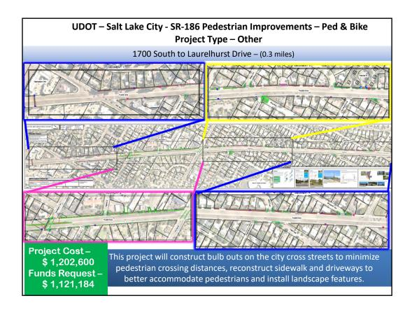
This project will provide an improved pedestrian experience by enhancing the parkstrip that separates the sidewalk from the roadway. This project will increase pedestrian safety by decreasing the crosswalk distance by the use of bulbouts. Driveways and sidewalks will be reconstructed to more easily accommodate pedestrians.
