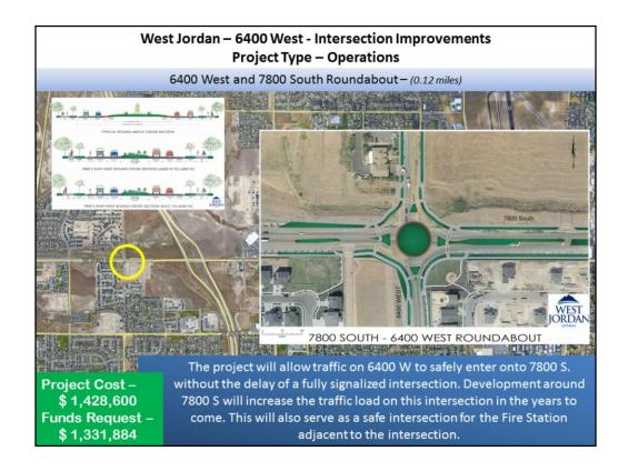
The project will allow traffic on 6400 W to safely enter onto 7800 S. without the delay of a fully signalized intersection. Anticipated development both North and South of 7800 S. will greatly increase the traffic load on this particular intersection in the years to come.
