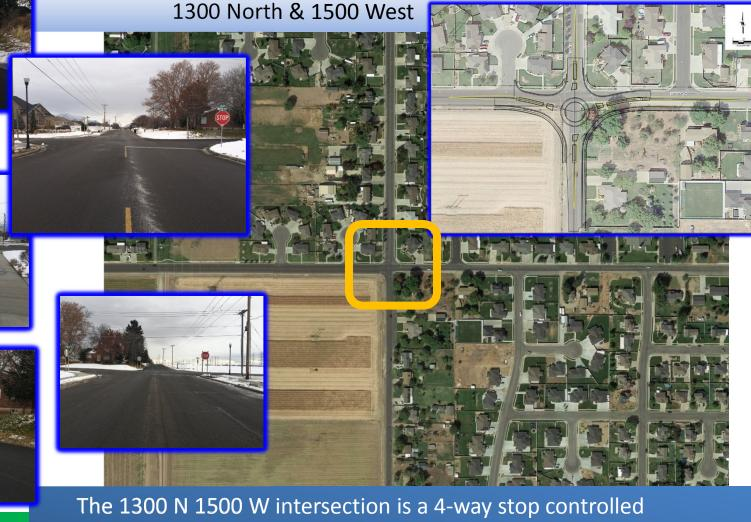
Project Cost – \$ 2,190,100 Funds Request – \$ 1,000,000 The 1300 N 1500 W intersection is a 4-way stop controlled intersection. Sight distance on the southeast corner is obstructed due a hill. The project would remove the obstructions and construct a roundabout at the intersection to improve safety, and mobility for pedestrians, bicyclists, vehicles, and improve air quality.
