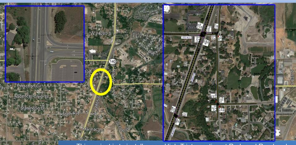
Project Cost – \$ 600,000 Funds Request – \$ 550,000 This project is to install a new High-T intersection at Redwood Road and 14600 South where the City is planning to extend 14600 South. Currently, the intersection of 14400 South and Redwood Road is functioning at a level service F and has large delays and significant safety issues due to the poor sight distance and geometry of the 14400 South and its connection to 1690 West and Loumis Parkway being less than 300 feet.
