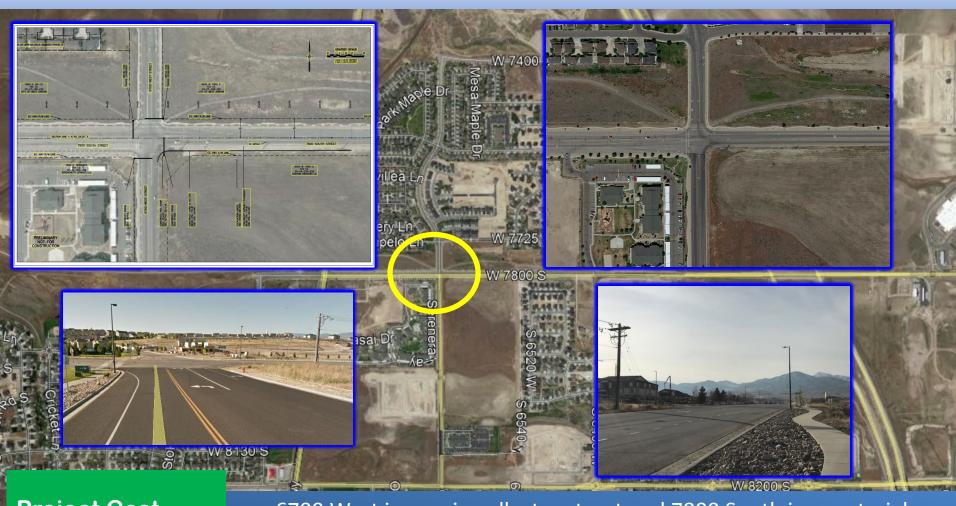
Project Cost – \$ 1,000,000 Funds Request – \$ 500,000 6700 West is a main collector street and 7800 South is an arterial street. This intersection is in a growing area and needs to be updated to handle the expected traffic growth. This project would replace the current stop controlled intersection with a signal or roundabout.
