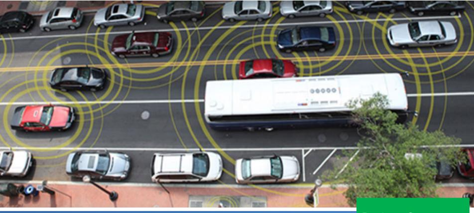
Connected Vehicles are about to fundamentally alter traffic management capabilities by allowing the communication of vehicles to vehicles and vehicles to infrastructure via short range radio. This initial project will continue to develop connected vehicle technology using vehicle to infrastructure systems to help maintain bus schedules. This technique is intended to allow a bus that is behind schedule to request an extended green light cycle in order to help the bus maintain schedule.
