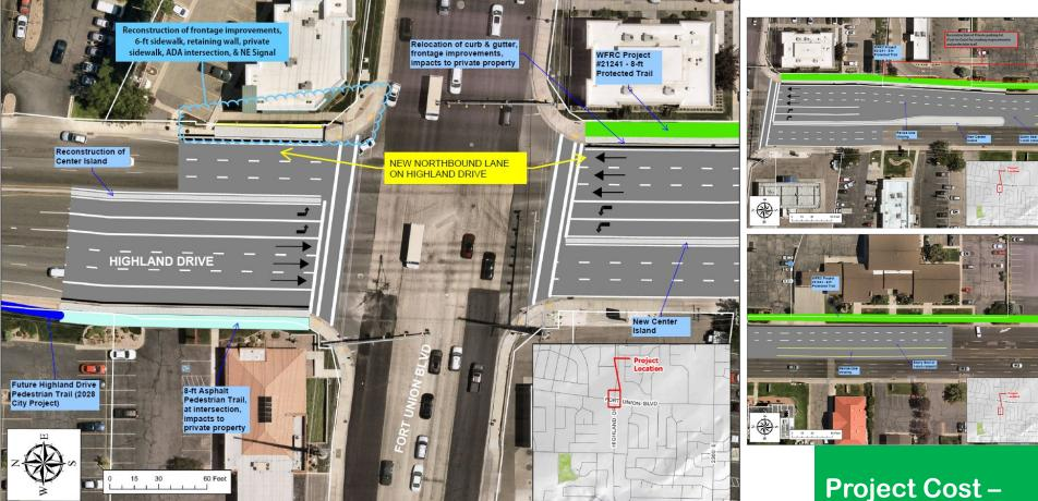
NB Highland Dr bottlenecks into two lanes at Fort Union Blvd, causing significant delays (74.7 sec/vehicle). The project will widen Highland Dr on the east side between 6990 - 7101 South, adding a third northbound thru lane to enhance capacity and traffic flow. Project Cost – \$ 3,825,000
