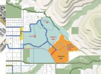
Improve visibility and connection between multi-use path and bike lanes on Wakara Way and Arapeen Dr. using green paint and visible markings. Consider a bike-and-ped scramble signal phasing. Concept may evolve based on TechLink TRAX design at this location. The TRAX station is anticipated to the east on Arapeen Dr.
