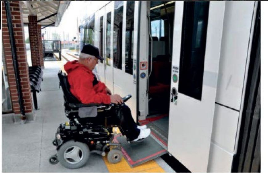
Low floor vehicles are wheelchair and walker accessible. New low floor vehicles will replace existing high floor cars.
