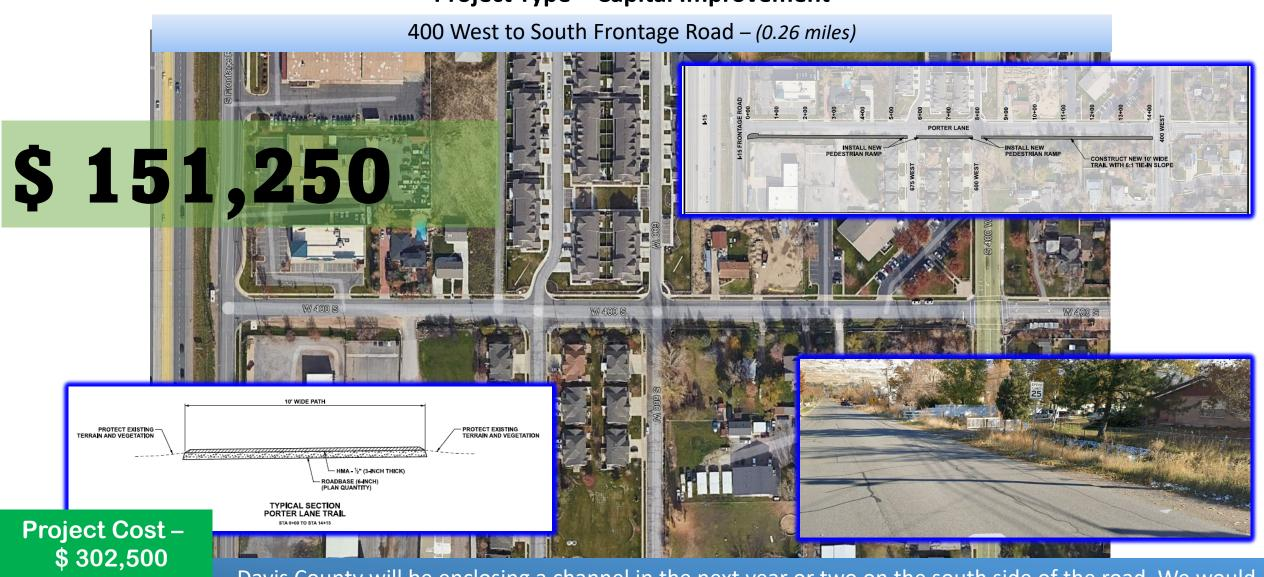
Funds Request – \$ 151,250 Davis County will be enclosing a channel in the next year or two on the south side of the road. We would like to put in a multi-use trail to connect 400 West to the Frontage Road on top of the enclosed channel.
