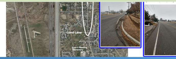
The proposed project is intended to improve drainage and add pedestrian facilities to the section of SR-106 (200 East Street) between Glovers Lane and Lund Lane on the east side of the road. The project includes acquiring right of way, storm drain, curb and gutter, sidewalk, retaining walls, and pavement widening.
