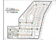
Figure 27. Example connectivity index calculation showing nodes and links. This example shows 22 links and 11 nodes which equates to a connectivity index of 2.0.
