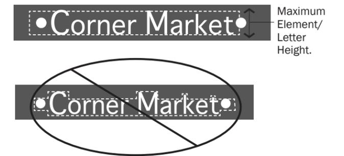
Figure 9.3 (2). Measuring Wall Signs.
