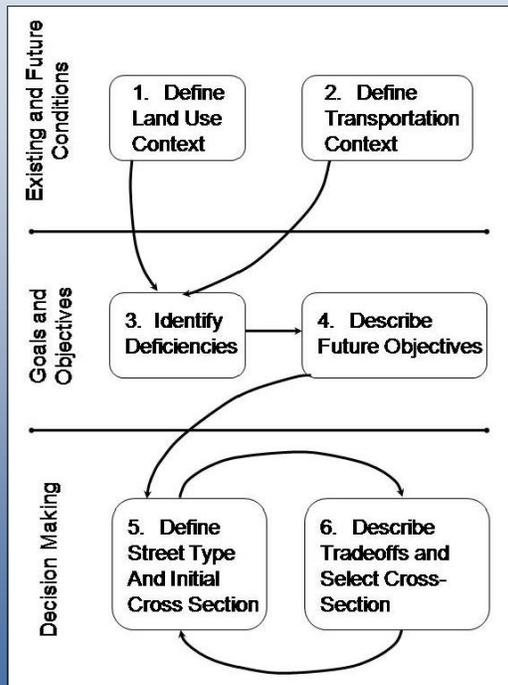
objectives as a guide to road design. Each facility segment is broadly assessed for its needs using the six step process outlined Figure 7-9.
